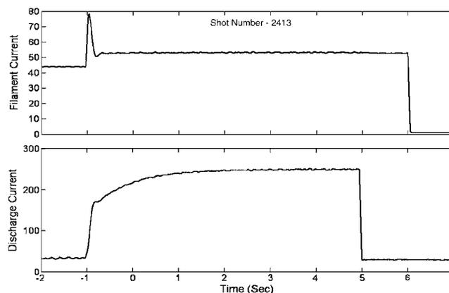
FIG. 10. Longer rise time in discharge current.
