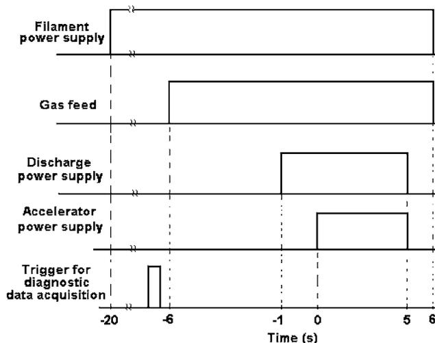
FIG. 3. Timing sequence for ion source operation.
